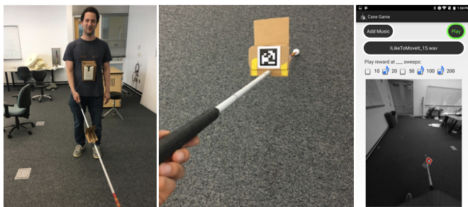
Figure 1: The prototyping environment we used to develop O&M educational games for students at Perkins School for the Blind. Left: the full system, including the harness to hold the phone and the tag to track the cane’s motion. Middle: a close-up of the April Tag affixed to the cane. Right: a screenshot from one of our prototype games running directly on the Google Tango Smartphone.
